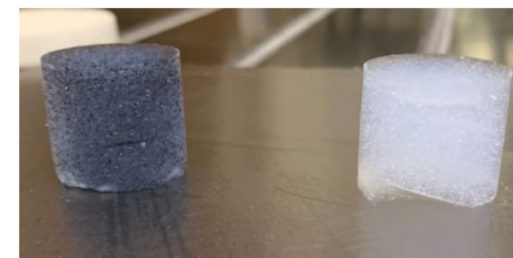
Figure 3: Carbon Burn Out Samples Before (Left) and After Heat Treatment (Right)
