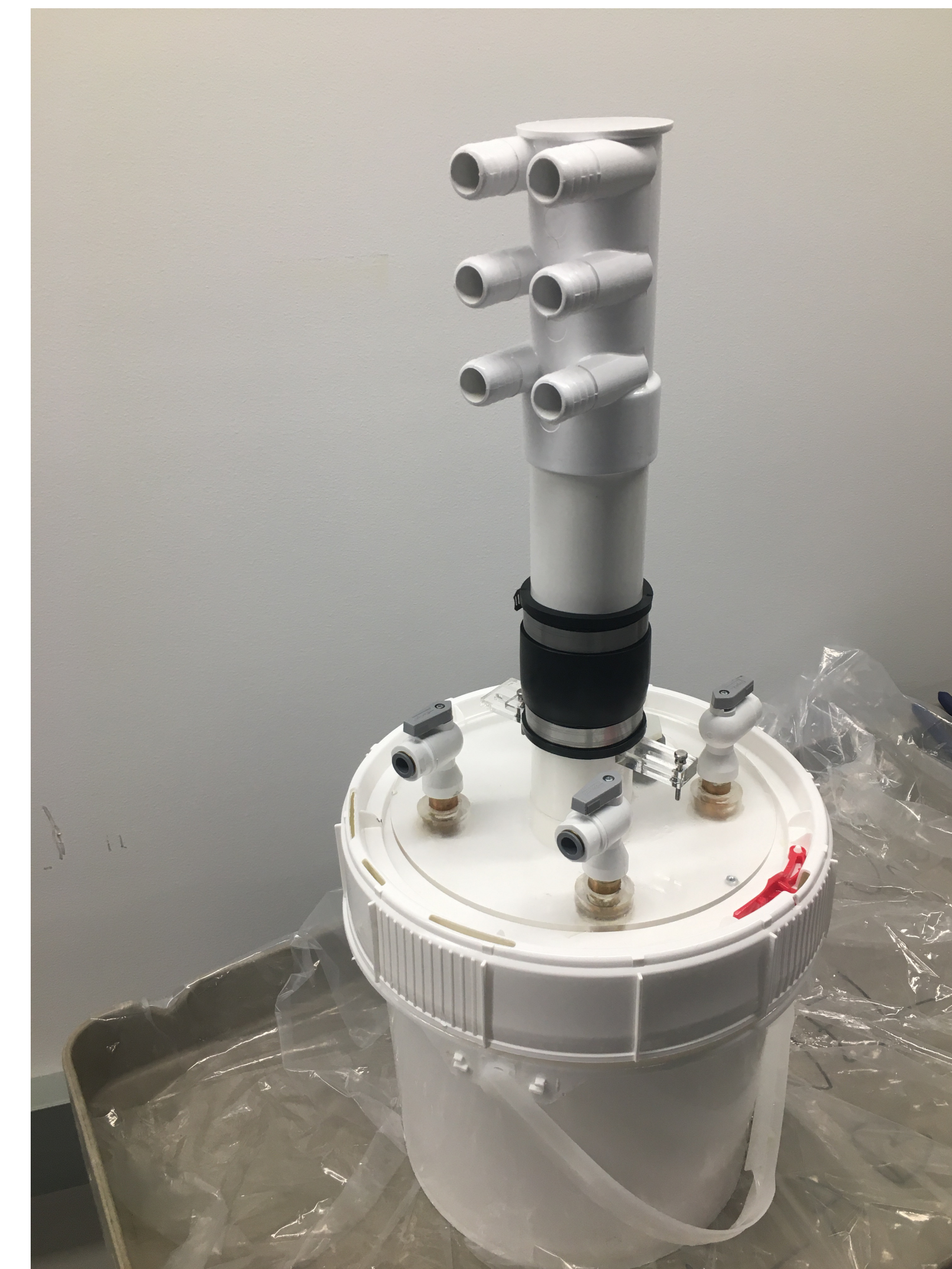
Figure 4: Laskin Nozzle aerosol generator fully constructed.
