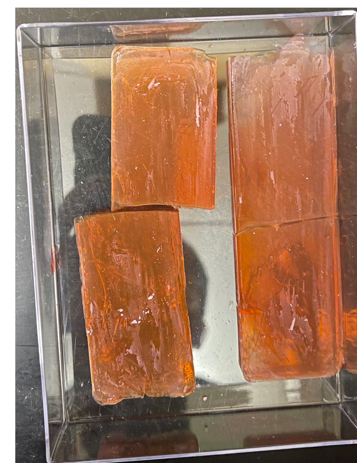
Figure 4. Rhodamine 6G dyed monolithic silica aerogels
