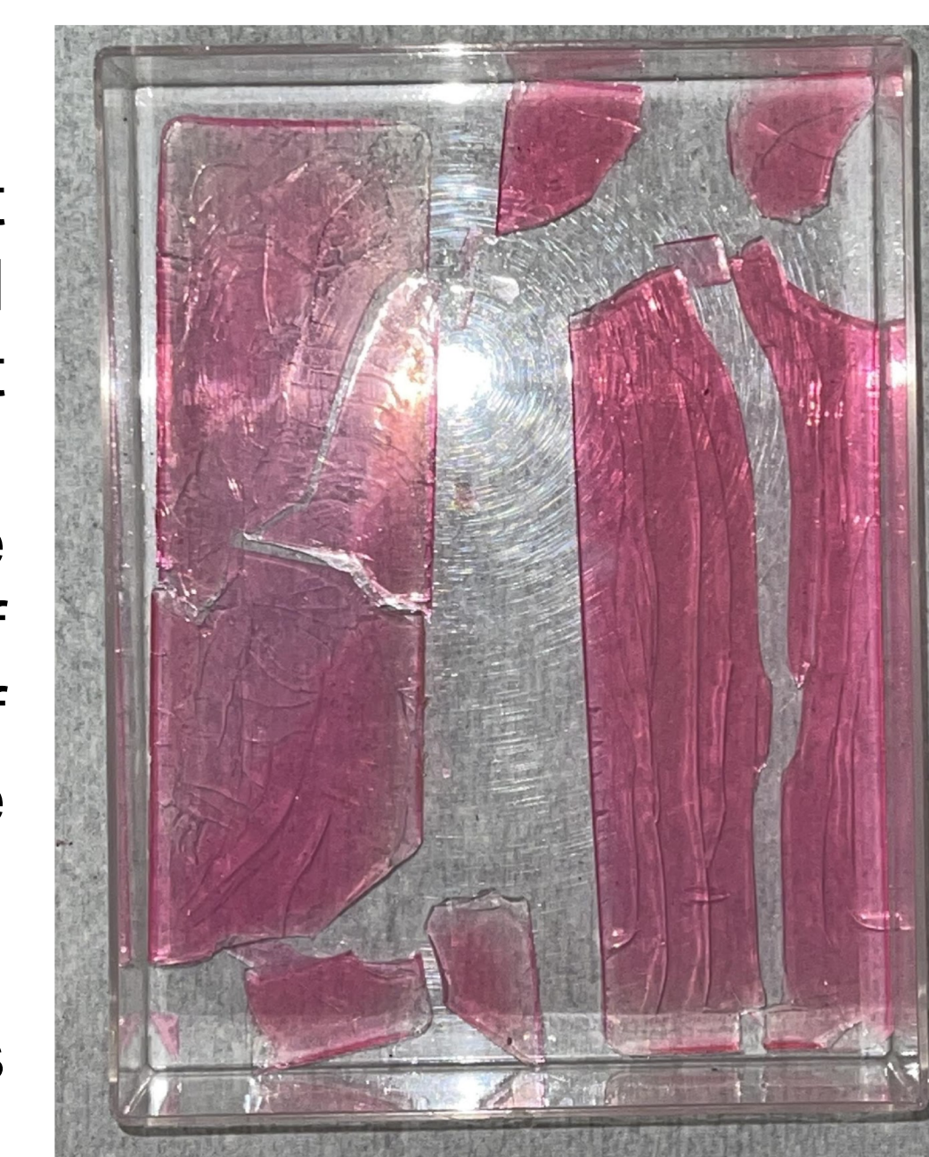
Figure 6. Rhodamine B successfully dyed into silica aerogel
