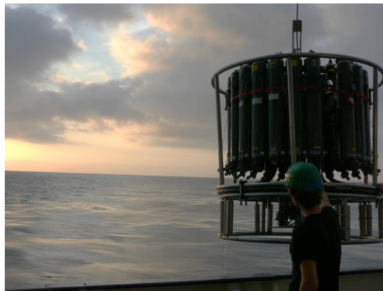
Deployment of CTD/Rosette from R/V Meteor off Peru. (Photo H. Bange, GEOMAR)
