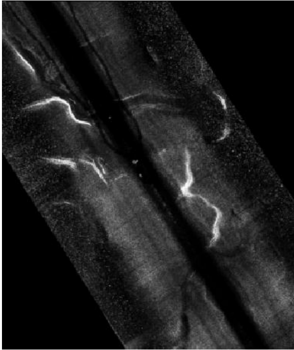
Fig. 16 TOBI run across the headwall area north of Agadir Canyon. Swath width is 6 km. Bright colors are areas of high backscatter.
