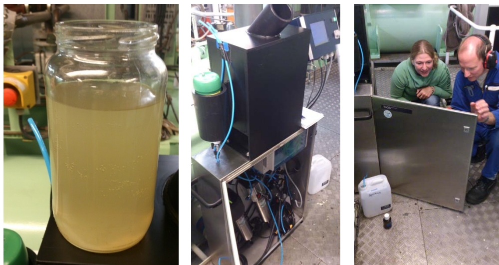
Fig. 33 Turbid sample water of the Maria S. MERIAN after treatment with bilge water separator (left); AquaPAK system with newly developed sensor and reference sensors, installed at the bilge water separator of the MSM (middle); briefing for operation of system (right).
