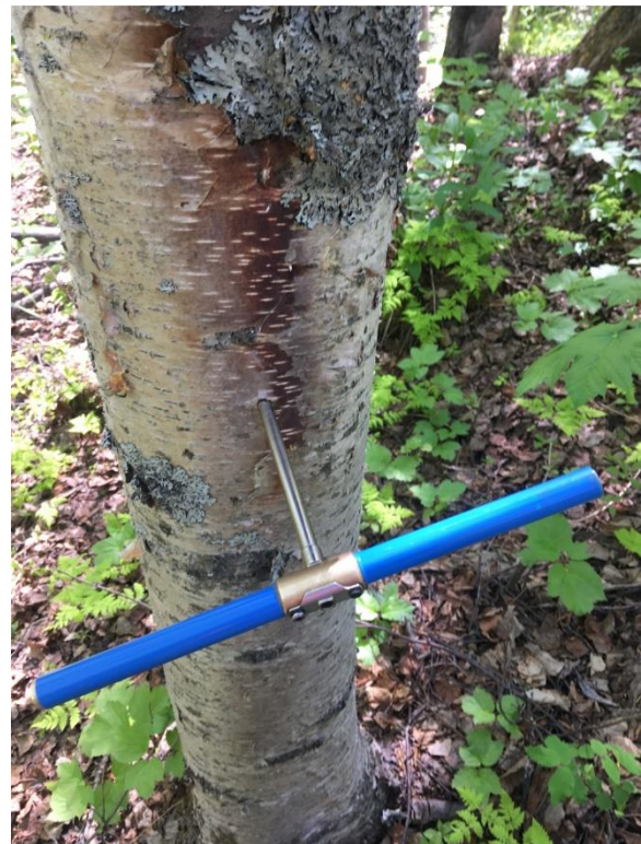
Figure 4. Increment borer in an Alaska paper birch with spoon and sample extracted.
