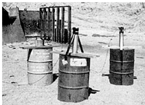
The implosion tube method of shocking rocks
