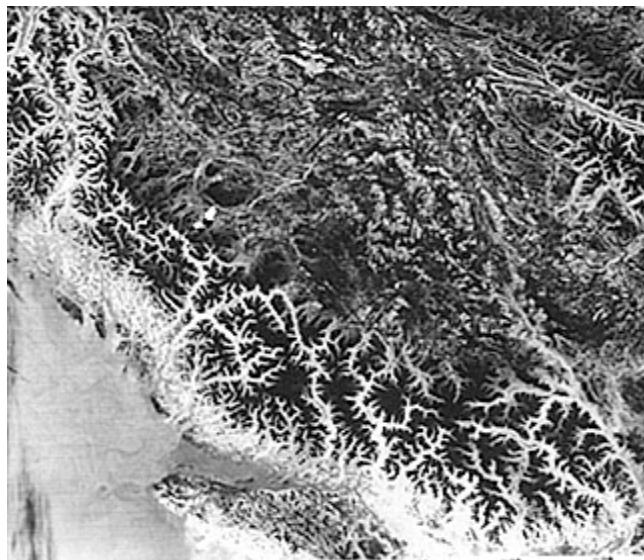
HCMM Night IR Image of British Columbia showing the different types of geomorphic terrains in the mountains
