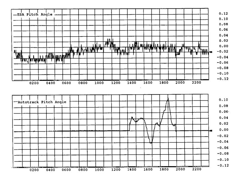
Figure 9. Typical pitch angle plot. Pitch is controlled by the ESA during the period of the Autotrack disturbance.
