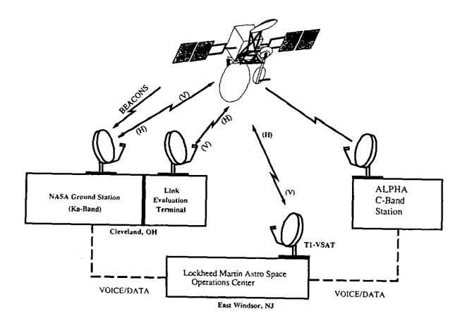
Figure 12. Ground stations used in initial on-orbit checkout of the ACTS satellite.
