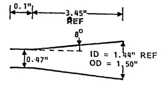
Figure 8 Transmit Scan Array Horn
