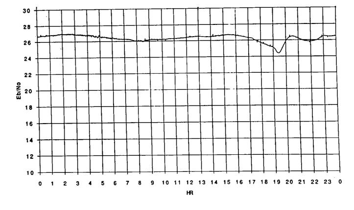
Figure 19 Typical downlink east beam received signal by a T1VSAT ground station as afunction of time of day.
