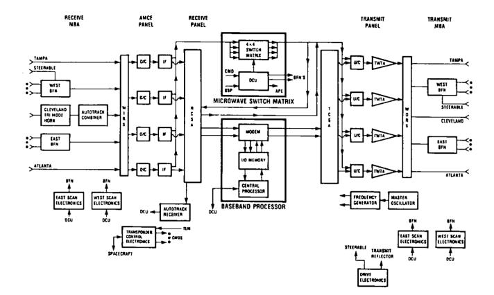
Figure 4. Block Diagram of the ACTS Communications Payload.
