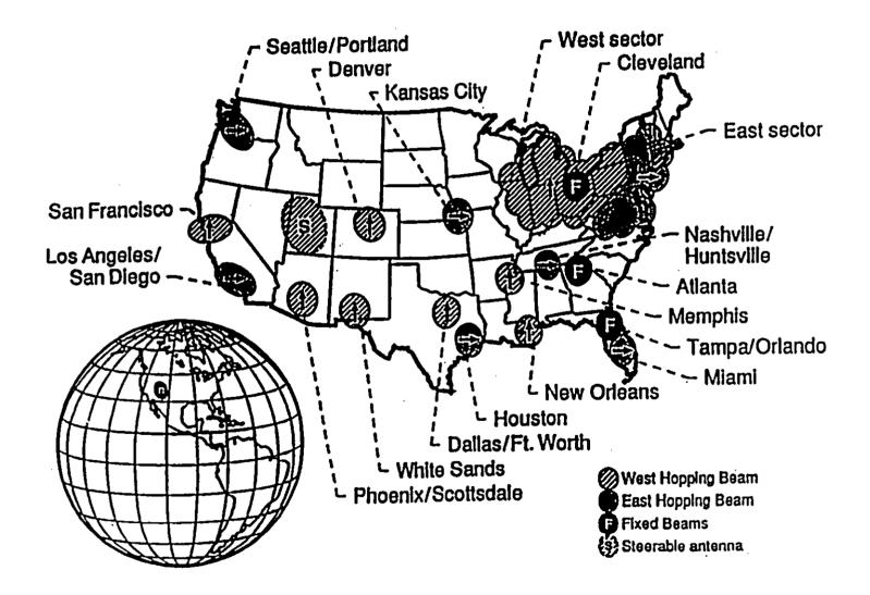
Figure 2 The ACTS Hopping Spot Beam and Steerable Antenna Coverage.
