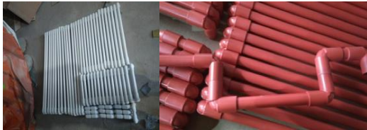
Gambar 4. Proses cat dasar dan finishing pipa PVC
