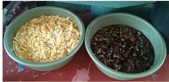
Figure-1. Fibers immersed with sodium hydroxide.
