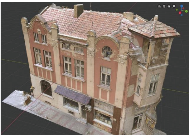
Fig. 14. Photogrammetric model produced by software ReCap (16) opened in Blender (11, 12)
