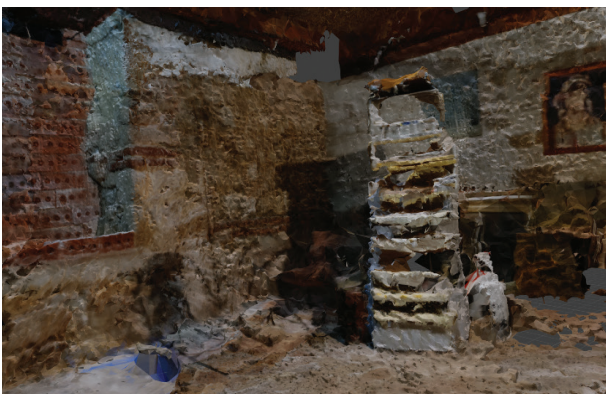
Fig. 15. Photogrammetric model of the interior produced by Meshroom (9,10)
