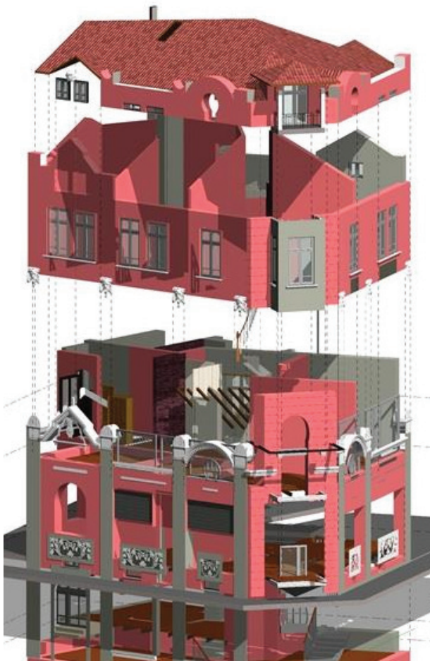
Fig. 22. Vertical displacement study of walls, wall construction, floor structure and layers, pilasters, ornamented decoration, mascarons, cornices.
