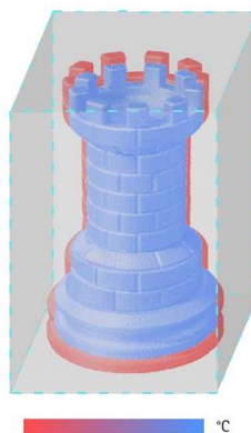
Figure 2.10 Shrinkage behavior of the part during cooling phase [8]
