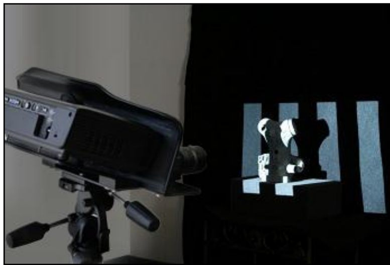
Figure 2.7: An object scan by using white light scanner (Tong, 2011).
