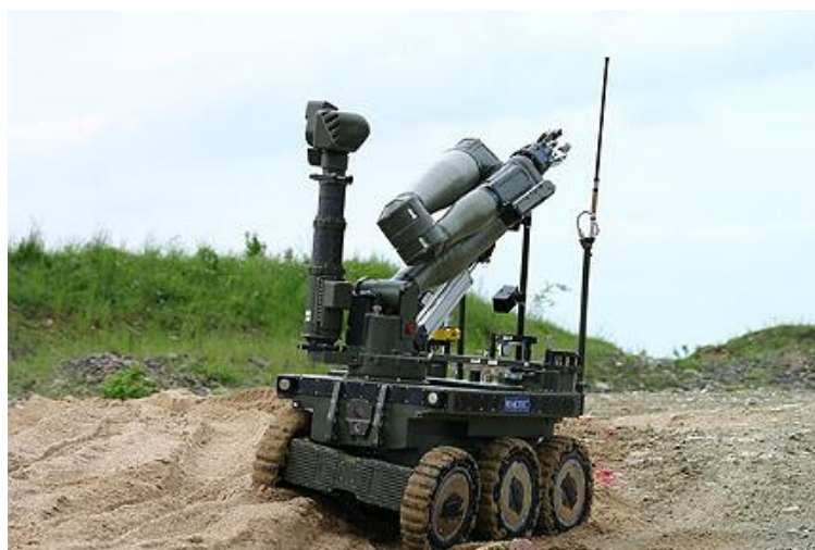
Figure 1.2: UGV: CUTLASS used for explosive ordnance disposal (EOD) missions
