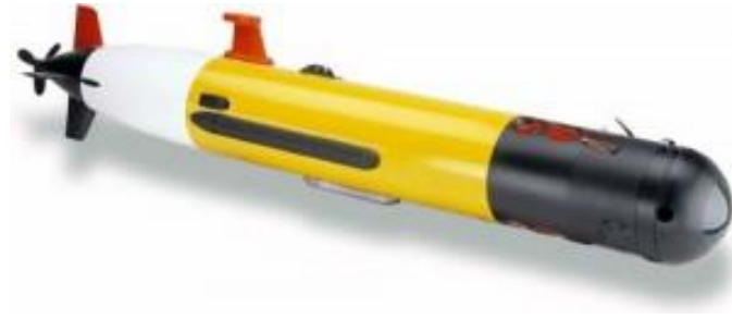
Figure 1.3: UUV: REMUS 100 applications include mine countermeasure, harbour security and debris field mapping
