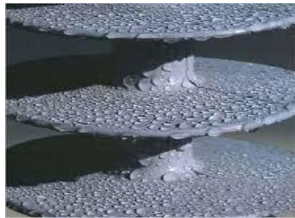
Figure 1.2: Water droplets on the polymeric insulator surface
