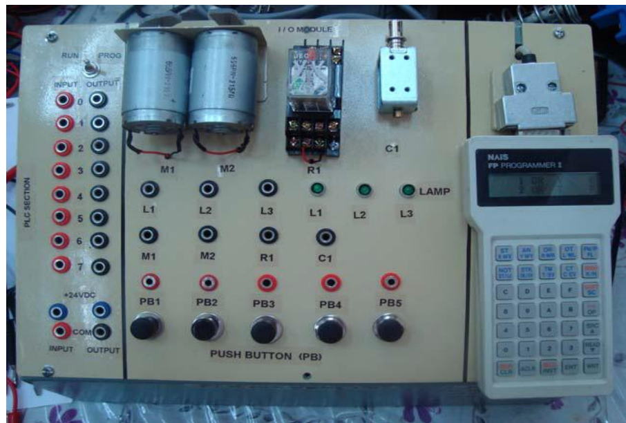
Figure 2.1: Overall view of PLC Kit
