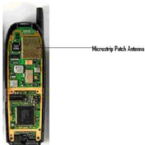
Figure 2.9: Patch antennas inside a NOKIA cellular phone
