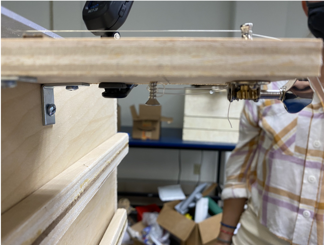
Figure 32: String Stop on The Vibration Station
