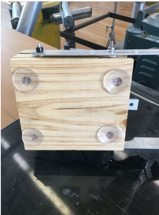
Figure 32: Bottom view of final prototype showing the suction cups
