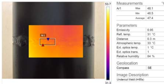
Figure-4. Infrared thermal image of undercut weld
