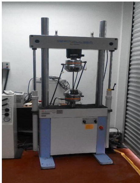
Figure 5. Universal tensile test machine with a high temperature chamber.
