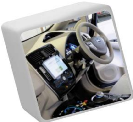
Figure 3: Smart Vehicle with driver assistant screen for safety message and infotainment message such as advertisement.
