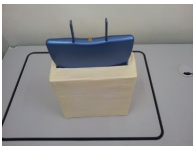
Figure 2: Modified Hyperlog antenna.
