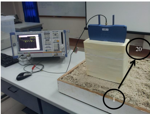
Figure 7: Scanning of GPR system.
