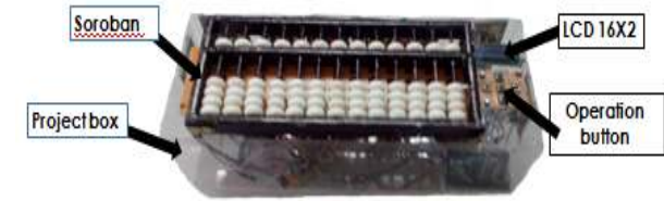
Figure 5: Parts of E-Abacus are fitted to the project box.
