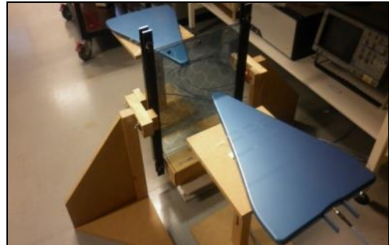
Figure 4. Measurement setup; Glass panels, antenna and wooden stands holding the panels
