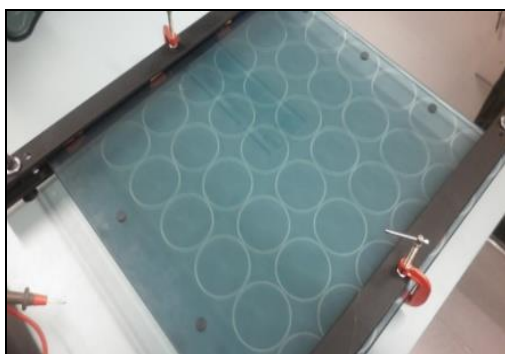
Figure 3: FSS prototype; the ring patterns can be seen on the glass surfaces
