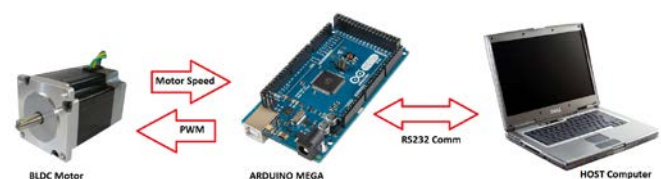
Figure 3 : Arduino Communication BLDC motor and computer
