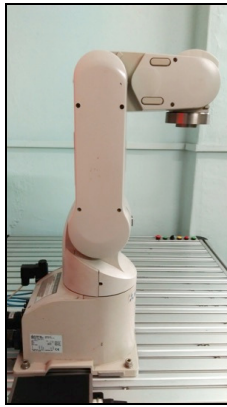
Figure 5: RV-2AJ robot with wrist pitch at vertical position.
