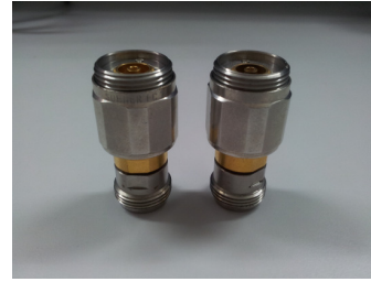
Figure 2: A pair of APC7 connectors is used for dielectric measurement.
