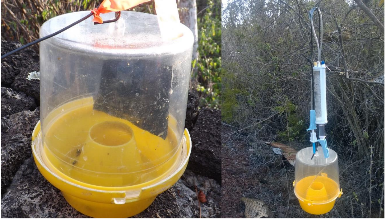
Figure 2. McPhail traps used in assays to extend the time of attraction of the solution with ethanol and acetic acid. a) CIPB inside the trap, b) IV drip system outside of the trap.
