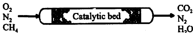
Figure 2.9: A Fixed bed Catalytic Reactor (Hayes & Kolaczkowski, 1997)
