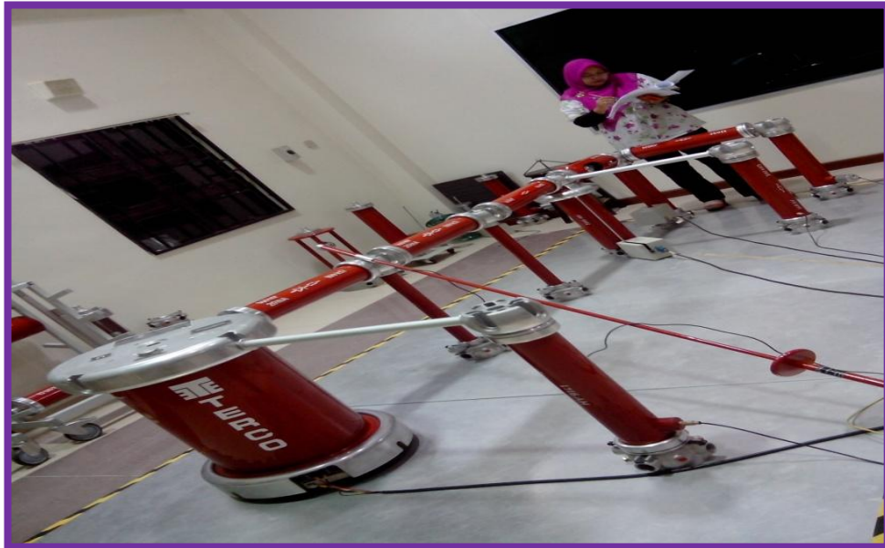
Figure 3.2 : The experimental setup of lightning impulse waveform in the HV laboratory
