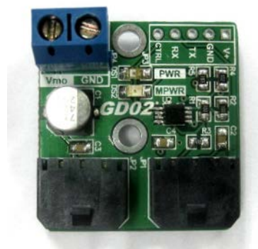
Figure 3.5: G15 serial servo driver
