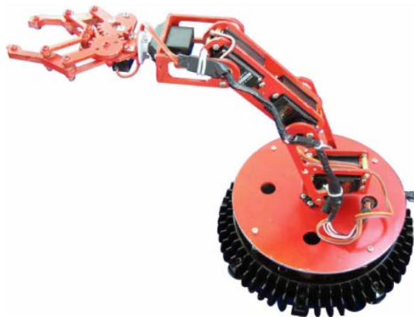
Figure 2.1: six-servo robot arm
