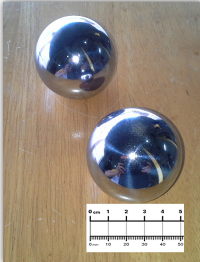
Figure 3.15 : Diameter of sphere's electrode
