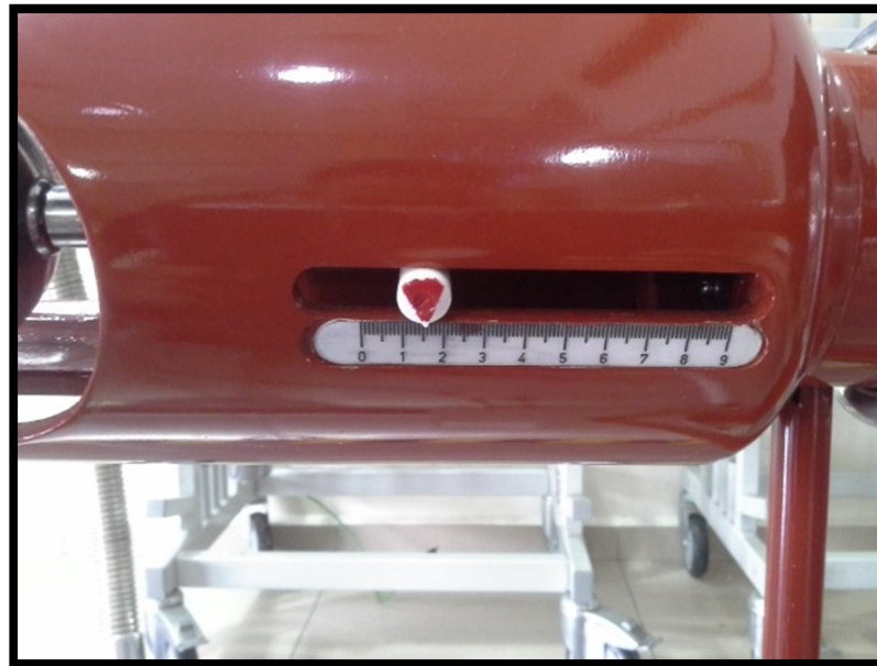
Figure 3.13: Measuring gap between sphere to produce Impulse Voltage
