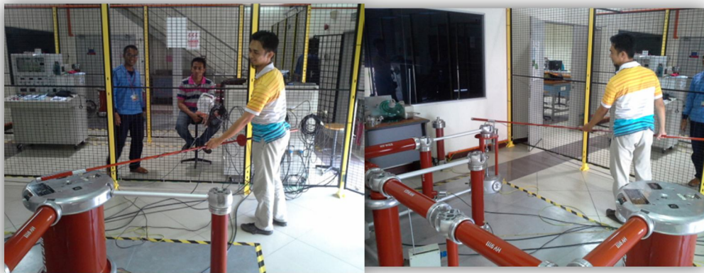
Figure 3.9: Grounding the component using earthing rod
