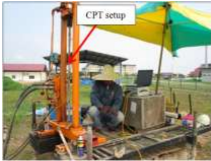
Fig.3: Cone penetration testing operation
