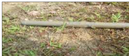
Fig.2: The tubular pipe pile model
