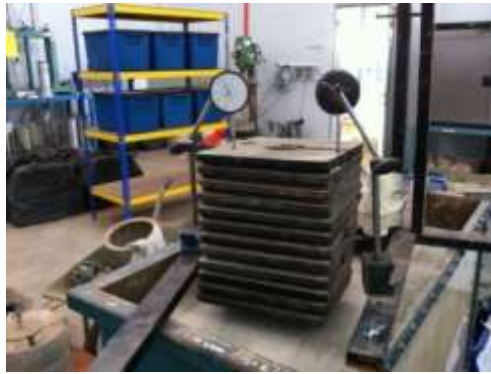
Fig. 2 Pile load test model
