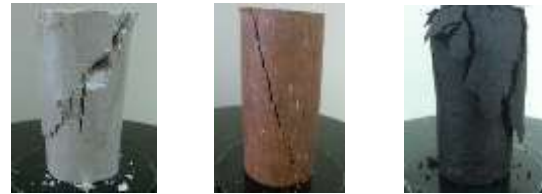
Fig. 4 : Failure patterns of UCS samples (a) Kaolin (b) Laterite (c) Parit Nipah Peat
