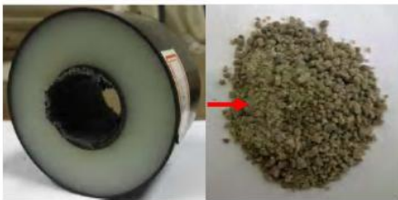
Figure 6 The recycle cross-link polyethylene, RPPW used as warm asphalt additive [37]
