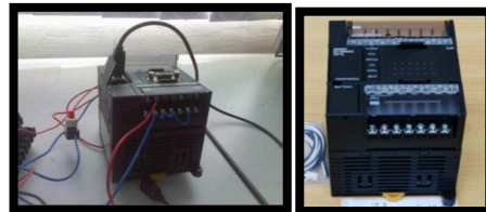
Figure 3: OMRON SYSMAC CP1L PLC
