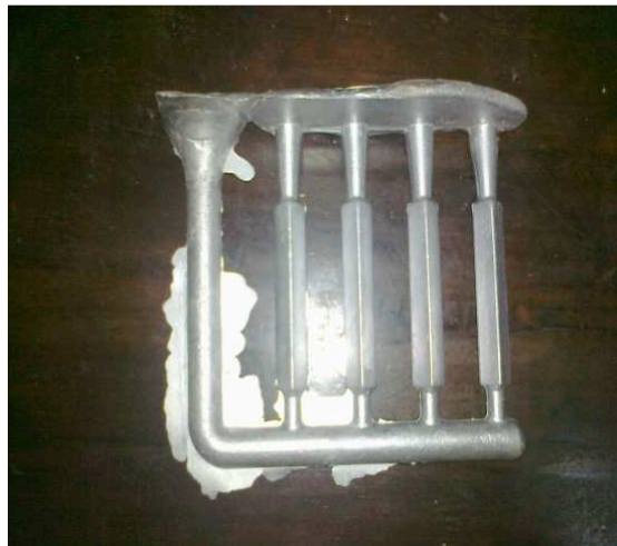
Figure1: Impact test specimen casting.
