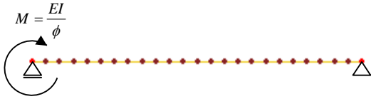
Figure 1 Plane beam in pre-loading state
