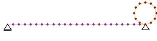
Figure 2 Plane beam in post-loading state
