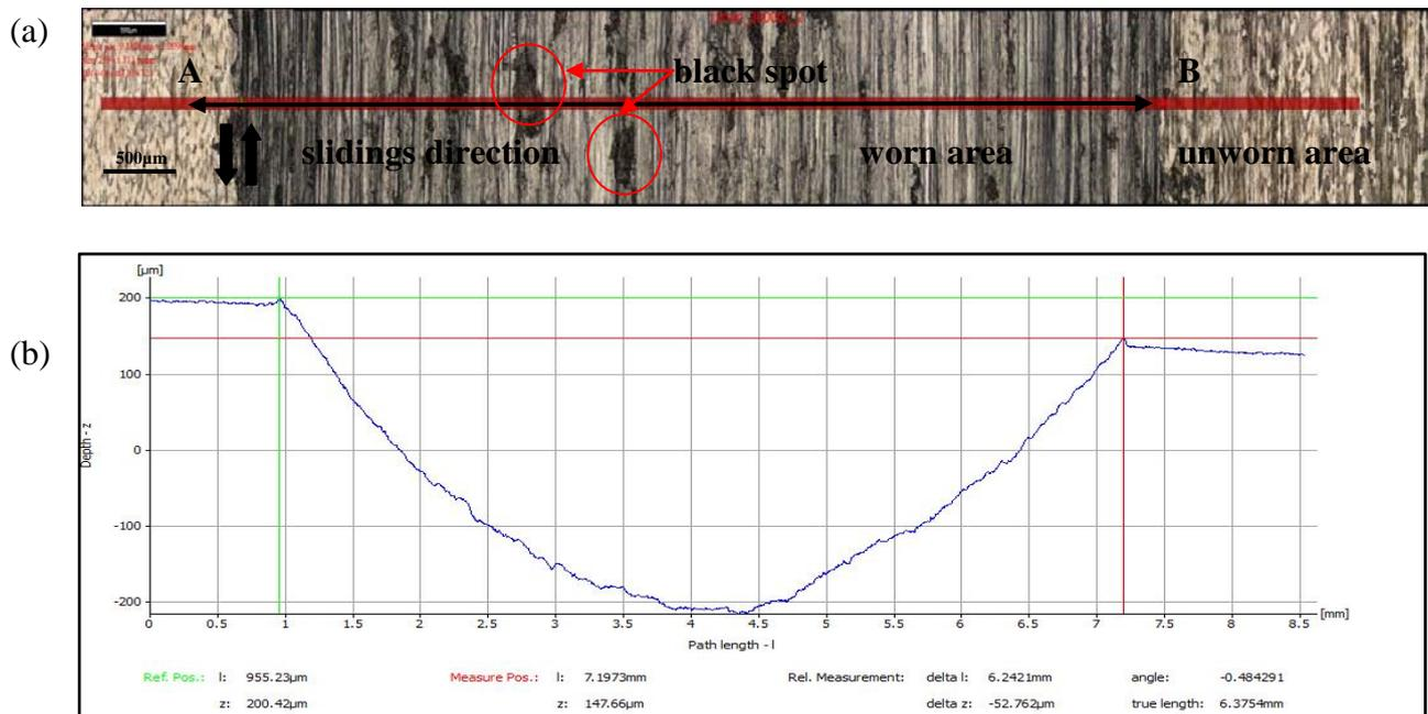
Fig. 3: Wear track profile for sliding until 12600 s (a) the plan view of the wear scar (b) The profilometry of the wear scar width and depth at middle track
