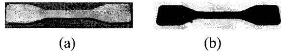
Fig. 6 Tensile strength sample from injection molding (a) Original ABS material (b) ABS-Iron material
