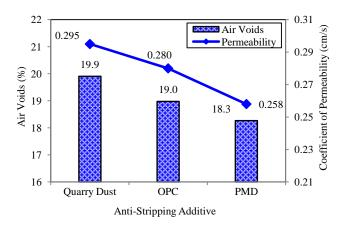
Figure 4 Result of air voids on coefficient of permeability
