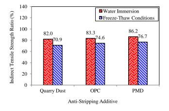
Figure 5 Comparison of ITS Ratio (ITSR) for PA mixes
