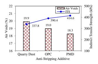
Figure 2 Effect of air voids on ITS for dry PA mixtures
