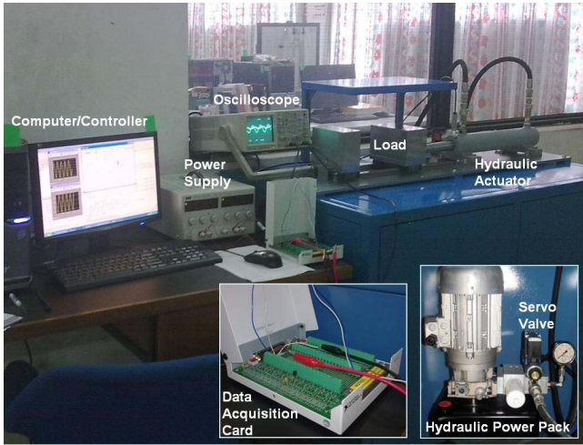
Fig. 3 Experimental workbench of EHA system
