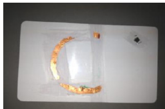
Figure 4: RFID Tag Antennas from Copper Etched
