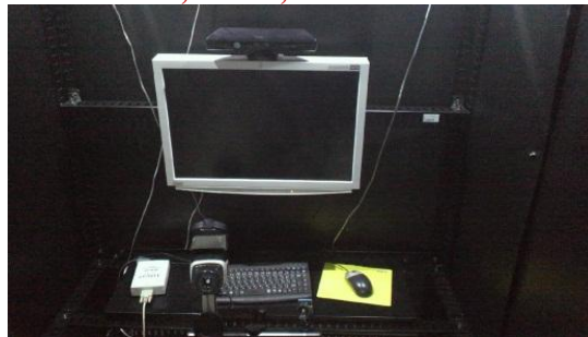
Fig.2. Camera setup (Thermal Camera (Right): NEC TH7800, Visual Camera (Left): USB CMOS Imaging Source DFK22AUC03 and Windows RGB-D camera (Upper))
