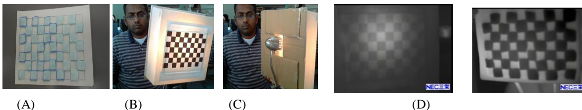
Fig. 2. (A) Chessboard attached with Fever Cold Plaster (back View), (B) proposed collaboration board attach with flood lamp, (C) Thermal image chessboard (light source 500 W, conventional chessboard), (D) Thermal image chessboard (light source 500 W, proposed Chessboard)
