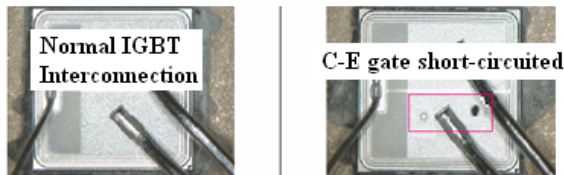
Fig. 11. De-capsulation Photo of the IGBT Switching Power Device
