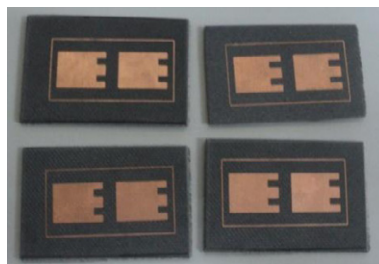
Fig. 4. Fabricated samples of dual gap on the rectangular patch element
