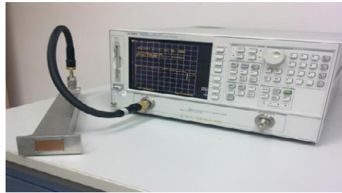
Fig. 5. Measurement setup for scattering parameters measurements
