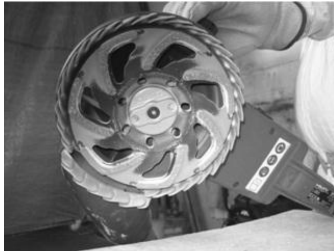
Figure 2.13: A 15 cm LEV grinder with vacuum system (Khanzadeh et al., 2007)
