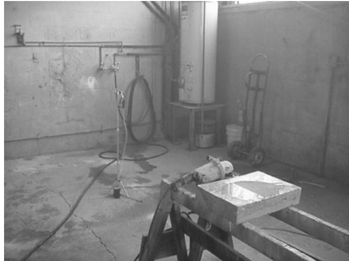
Figure 2.12: A 17.5 cm size wet grinder with water hose attached (Khanzadeh et al., 2007)
