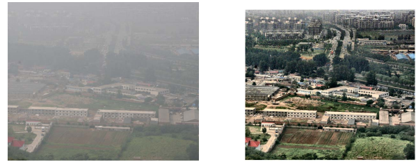
(a) Input image (b) Output image Figure 3. Removing fog using dark channel prior [53]
