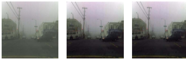
(a) Original image (b) SSR output (c) MSR output Figure 3. Results from Retinex algorithms [43]
